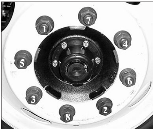
Lug nut tightening sequence.
